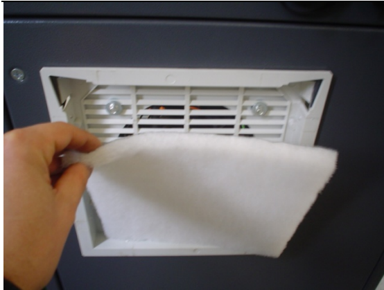
Figure 67: Checking and replacing the dust filter
