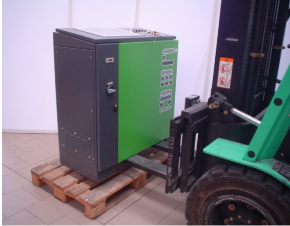
Figure5:Electrical Cabinet move with forklift 用叉车移动电柜
