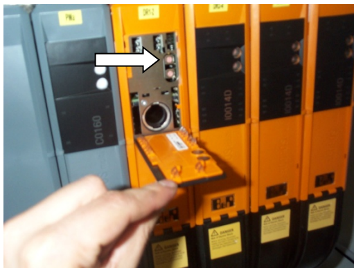
Figure 90: Replacing a drive 更换驱动器
